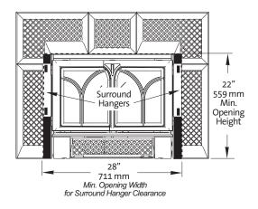
Figure 3. Minimum opening clearance. Optional Lattice Surround shown.
